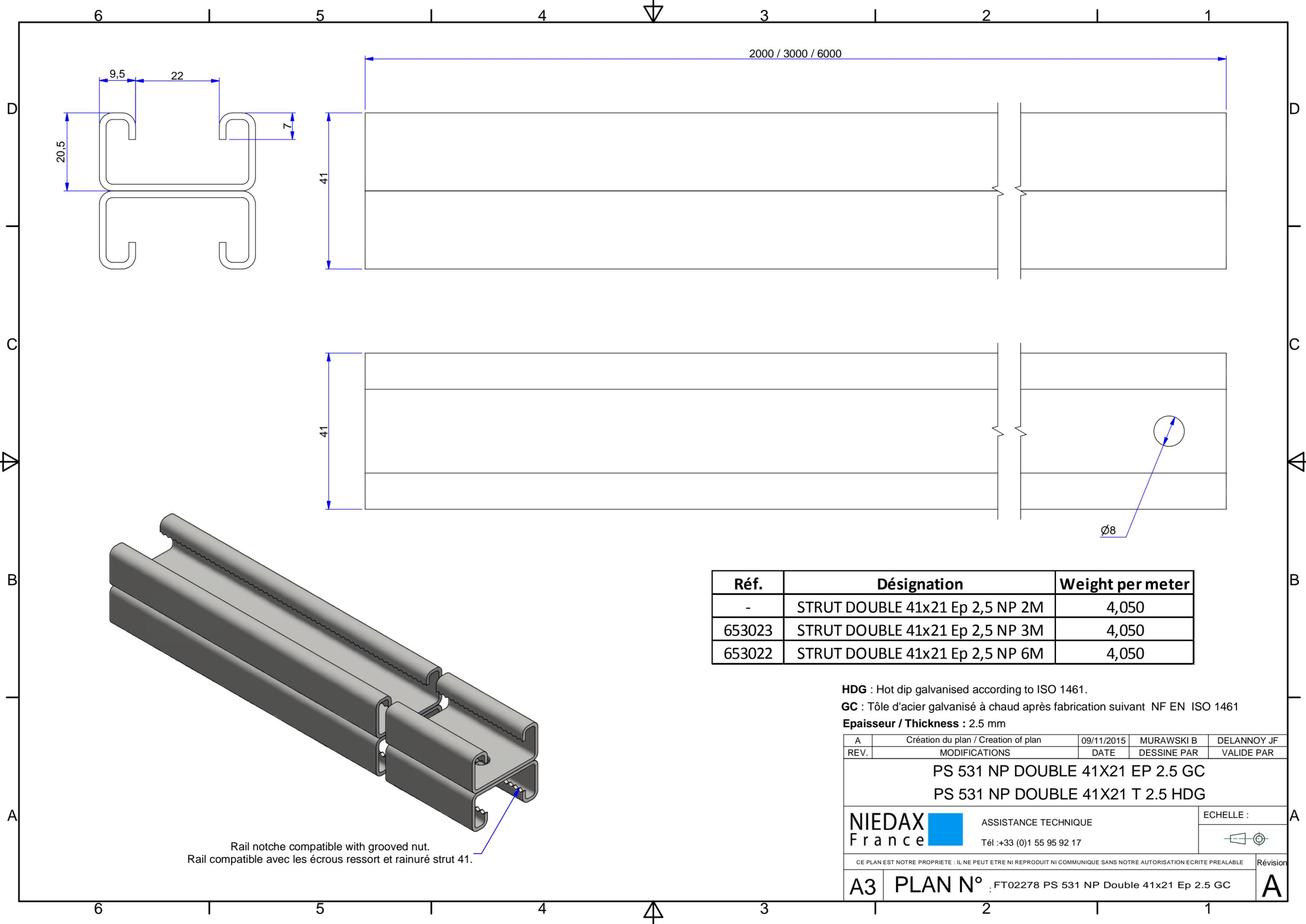
Rail notche compatible with grooved nut.
